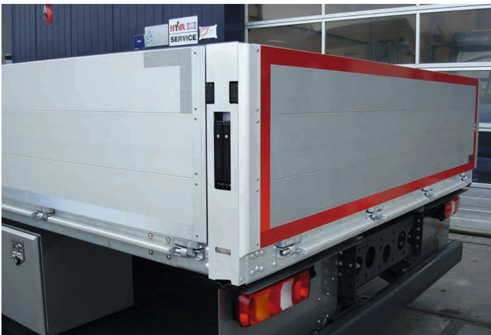
HESTAL SolidMaster 802 dropside pillars in 600mm (microZINQ®coating)
