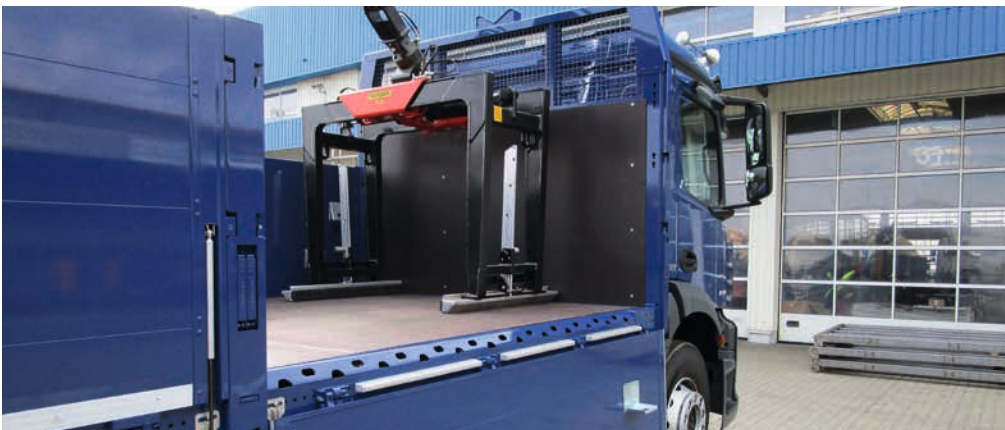
HESTAL SolidMaster 802 dropside pillars in 1,000mm with double locking (KTL and powder coating)
